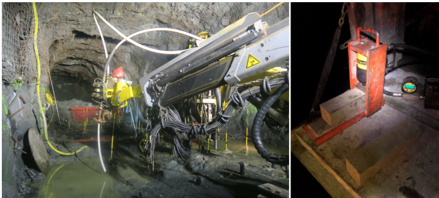
Figure 1: Setup for pull out tests on single 7 strands steel cables (5/8") and end-beam tester on 3"x3" grout samples.
