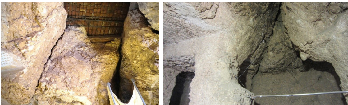
Figure 2: Wedge in the roof of tomb TT95 (left) with remains of the final tomb painting indicating the final designed roof location (middle left side) and (right) the displacement sensor placed between the pillar with the through going fracture and an intact pillar, as well as wires for 10 temperature sensors.
