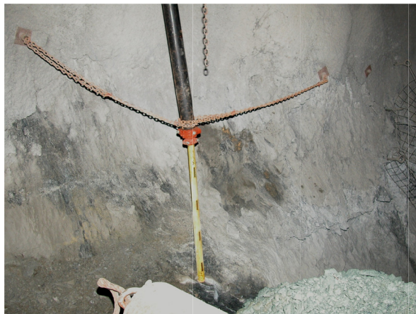
Figure 13 - A spraying and dumping setup
