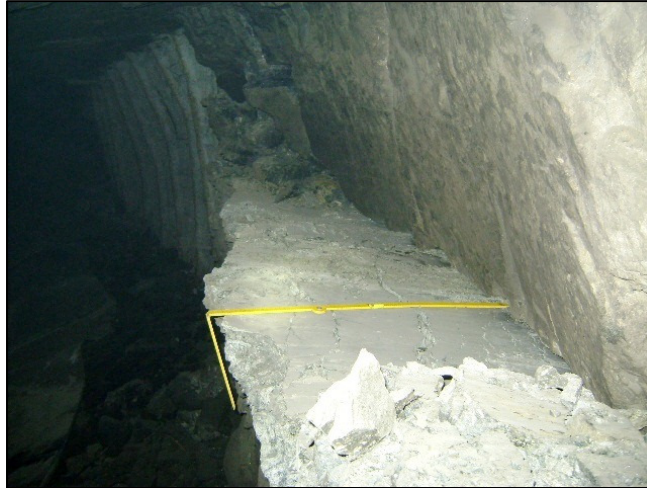
Figure 4 - Deformation of 75 cm along weathered pyroxenite layer
