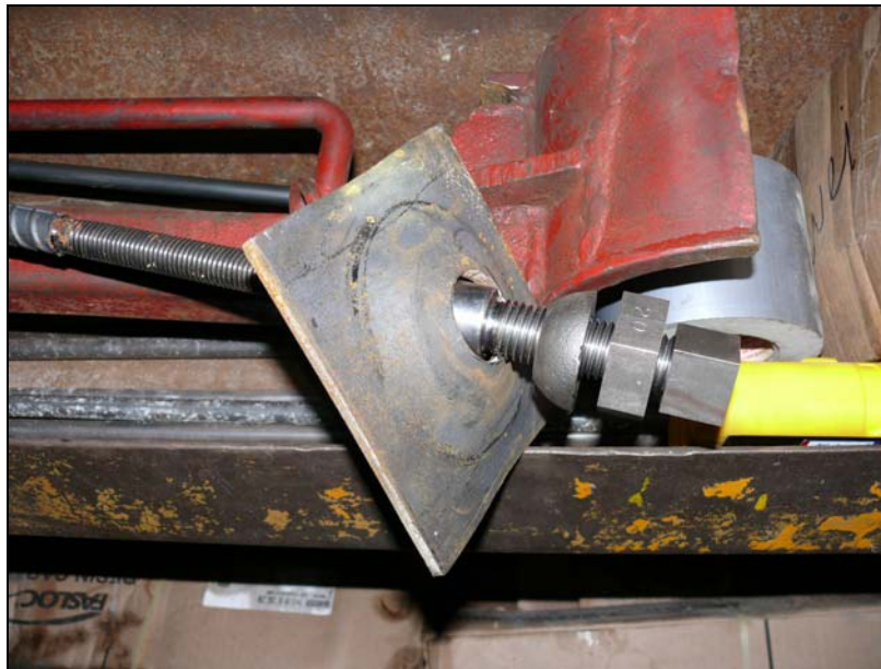
Figure 6 - Demonstration of a U-cell attached to a rebar
