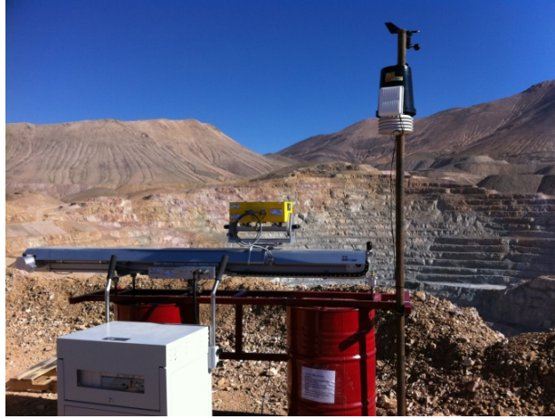
Figure 1 – Example of an open installation of a ground-based interferometric SAR for slope monitoring in an open-pit mine
