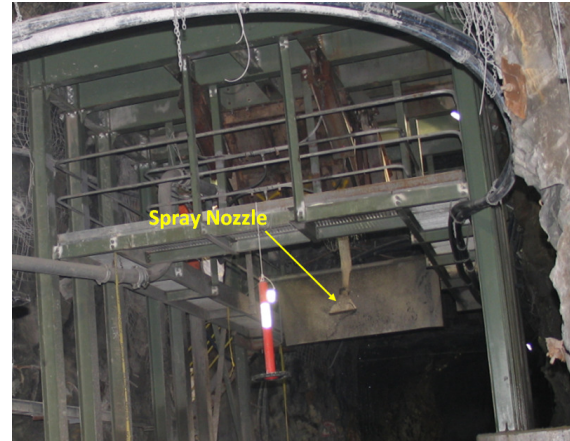
Figure 12 - Slurry spray at the load out station
