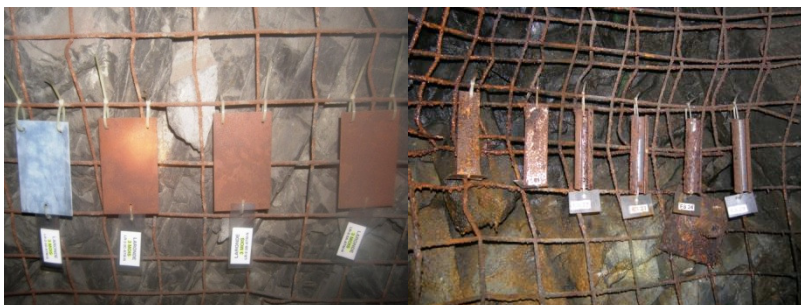
Figure 3 - Corrosion coupons attached to the mine screen on the drift wall, after a three-month exposure
