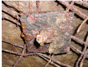
Figure 2 - Visual corrosion level chart (Dorion and Hadjigeorgiou, 2008)
