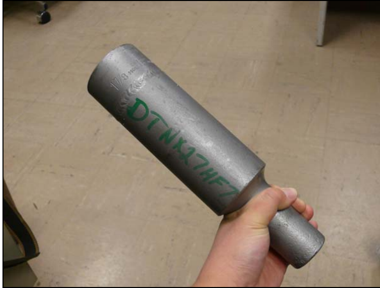
Figure 5 - 1 7/8 inch dolly for U-cell installation
