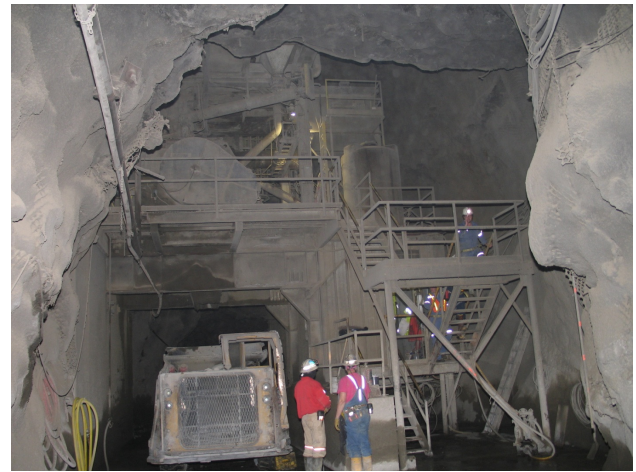
Figure 9 - An underground CRF batch plant
