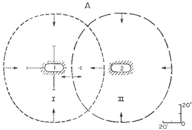
II = Second stress relief creep zone around room No. 2 shortly after mining room No. 2. "Negative" movement of the 10 ft. pin (room 1) for two days.
