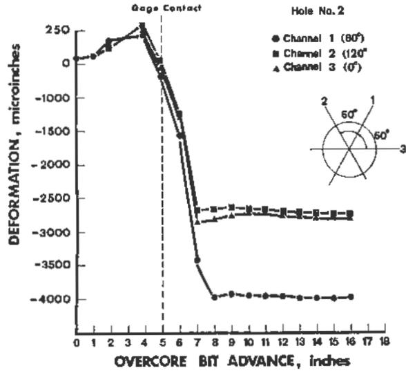
Figure 15. Typical overcoring stress-relief deformation pattern
