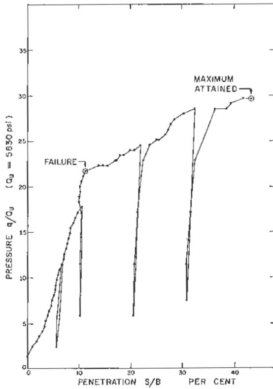
Figure 4. Pressure-penetration curve obtained in test B-18 (Indenter diameter:  $B=0.50$  in; depth of embedment:  $D_o=0.665$  in;  $D_o/B=1.33$ )
