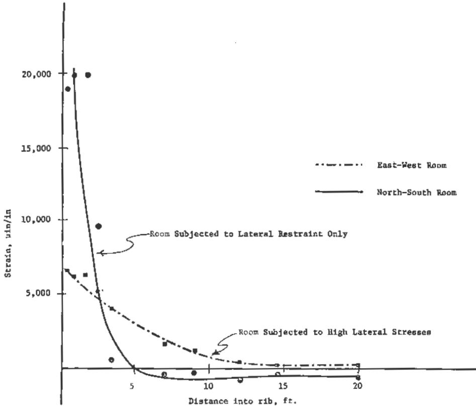
Figure 9. Pillar strains for rooms subjected to high and low lateral stresses.
