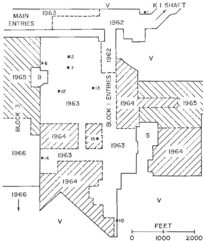
Figure 7. Mining sequence and location of closure measuring sites in blocks 1 and 3, K 1 mine, INC. Numbers of measuring sites correspond to creep curves in Figure 8.
