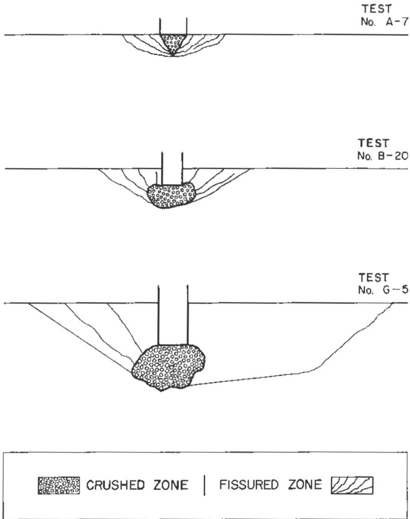
Figure 3. Types of failures observed in the tests
