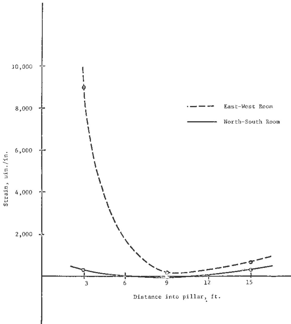
Figure 3. Pillar strains in a pillar of B-11 section in development.
