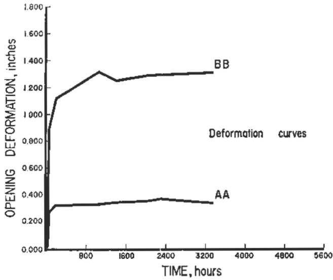
Figure 12. Time versus closure - station SS-7
