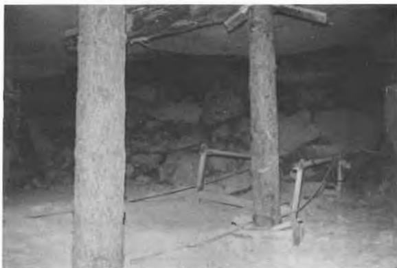
Figure 1b. Failure of all artificial support measures by steadily progressing roof fall.
