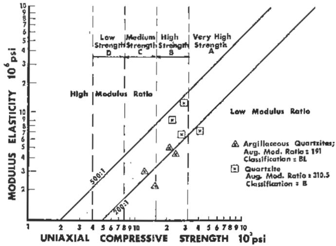
Figure 14. Uniaxial compressive strength versus modulus of elasticity
