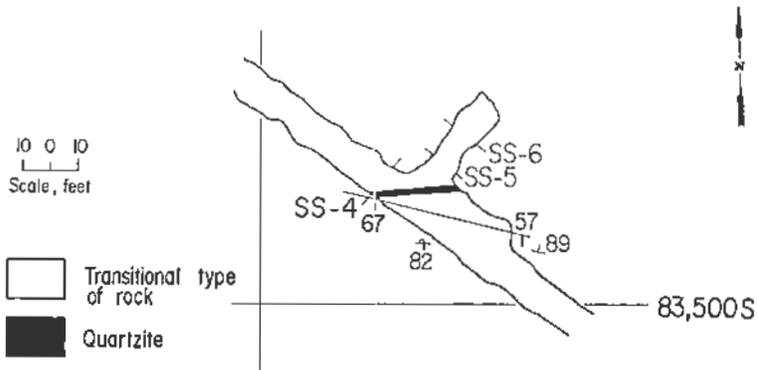
Figure 5. Detailed geology - overcoring site, stations SST-1 and SST-2
