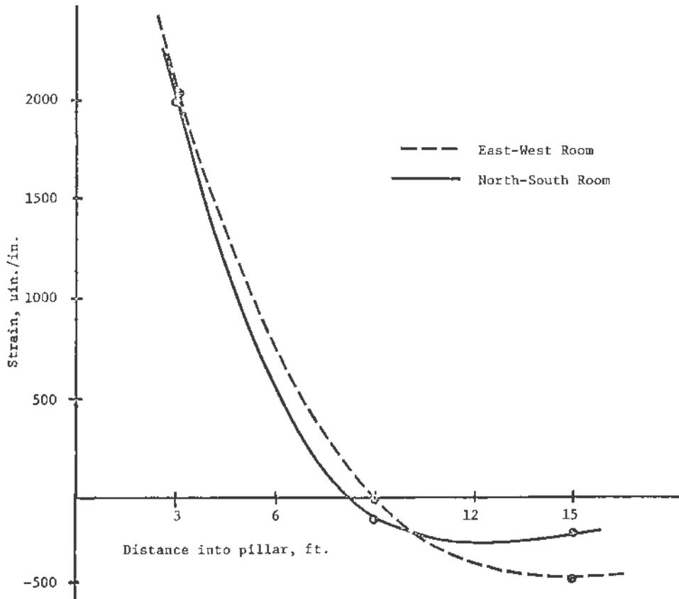
Figure 4. Pillar strains in a pillar of B-11 section in retreat.
