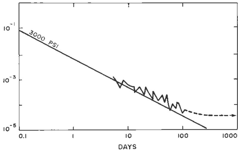
Figure 3. (Coolbaugh 1967) Predicted and measured opening closure rates at IMC.
