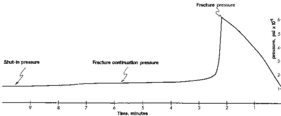
Figure 6. Pressure curve from hole No. 4 at 97 feet into the floor (sandstone formation).
