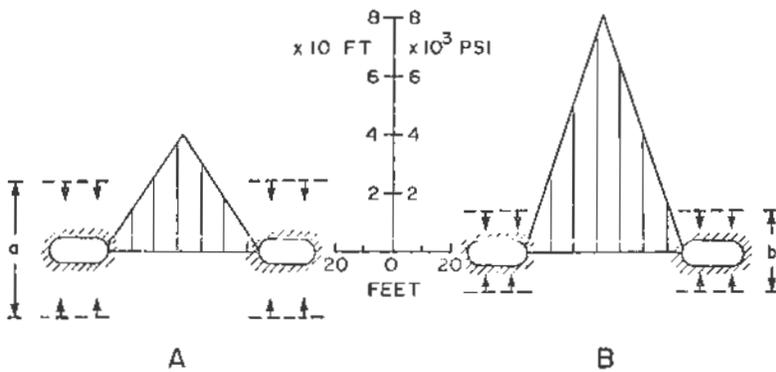
Figure 9. Development of pillar loads and vertical dimensions of creep zones around openings in carnallitic potash in mined-out areas at IMC.
