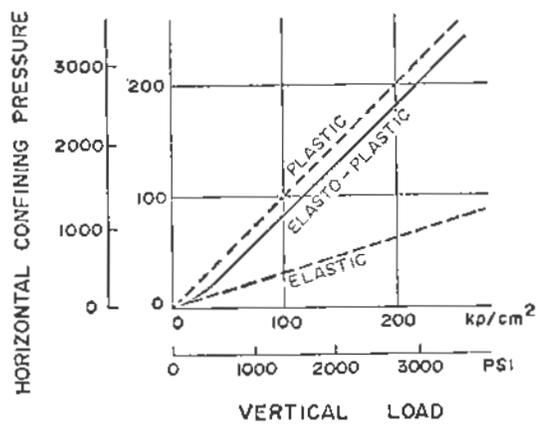
Figure 1. (Dreyer & Borchert 1955, Dreyer 1967) Elasto-plastic reaction of rock salt to vertical loading and unloading. Horizontal deformation is prevented by confinement. The calculated octahedral shearing strength increased from 50 psi under 285 psi to 75 psi under 3700 psi vertical load.
