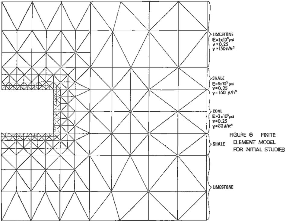
Figure 8. Finite element model for initial studies.
