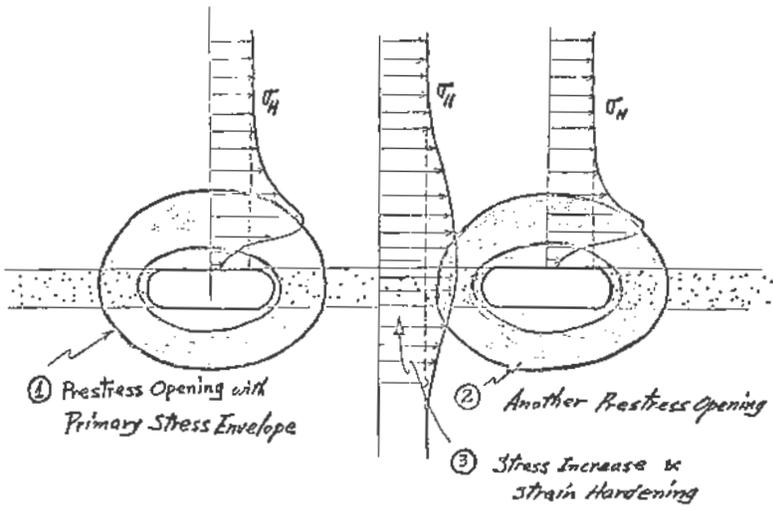
Figure 6a. Stress control method. (Step 1)
