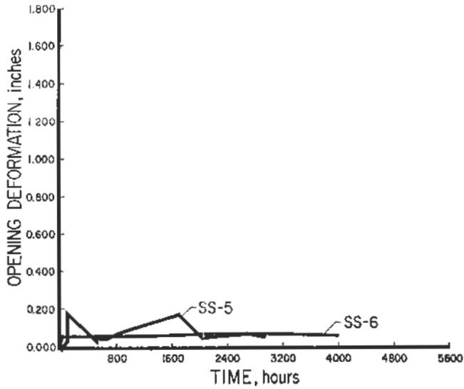
Figure 11. Time versus closure - stations SS-5 and SS-6
