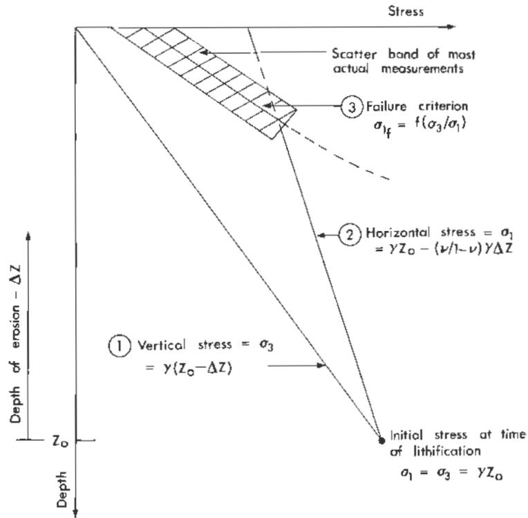
Figure 3. Loci of vertical and horizontal stresses as a function of erosion.
