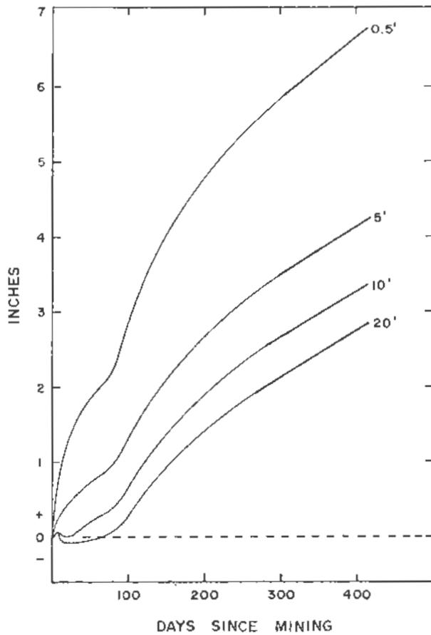
Figure 4. Horizontal movement of points at various depths in a 52 ft. wide pillar between two rooms in potash at 3,140 ft. depths. Openings cross-section 21 x 7.5 ft. For mining sequence see Figure 5.
