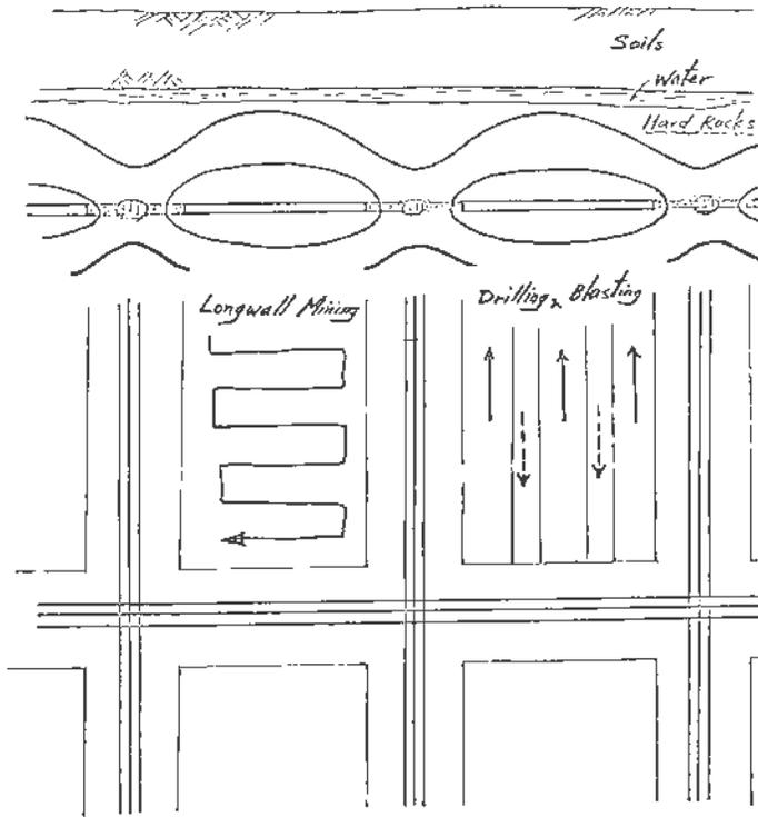
Figure 8c. Stress control for total extraction.
