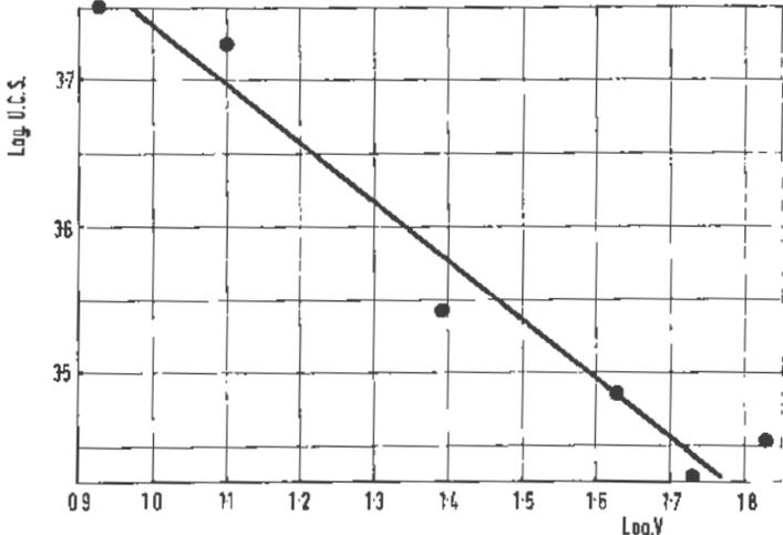
VARIATION OF COMPRESSIVE STRENGTH OF GYPSUM AS SPECIMEN VOLUME INCREASES
