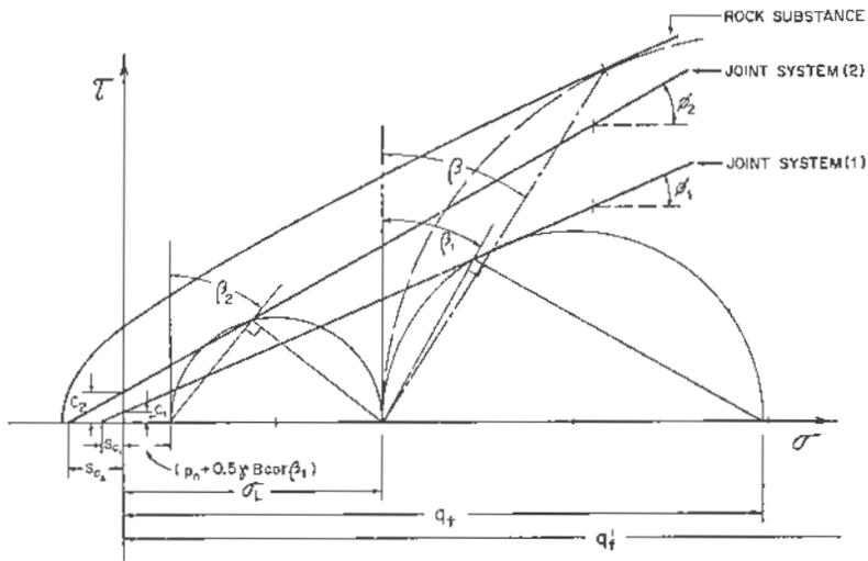
Figure 9. Graphical method for lower bound bearing capacity determination in jointed rock
