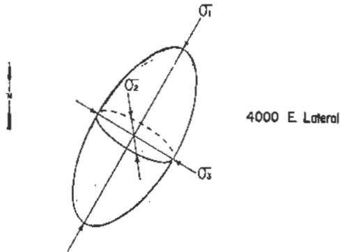
Figure 16. Stress ellipsoid
