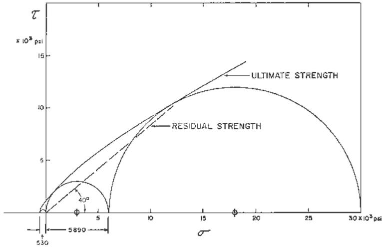
Figure 1. Ultimate and residual strength of carbonatite
