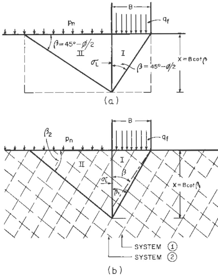
Figure 8. Stress fields (a) for homogeneous, and (b) for jointed rock mass
