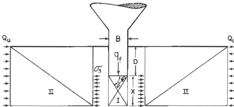
Figure 7. Stress fields for lower bound indentation analysis
