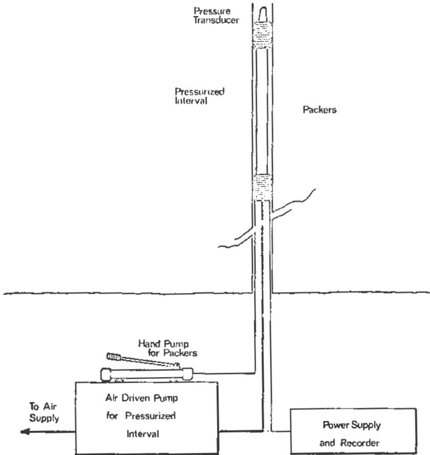
Figure 5. Hydrofac equipment and set-up.
