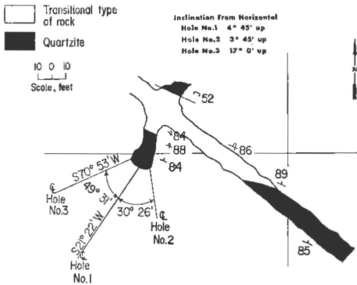
Figure 6. Detailed geology - stations SS-4, SS-5 and SS-6
