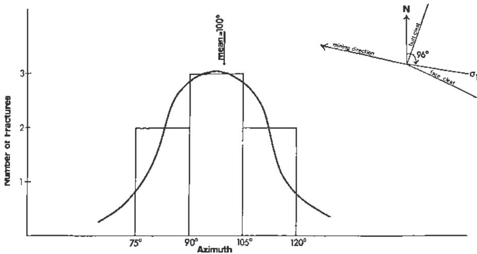
Figure 7. Stress measurements by the hydrofracture method. Histogram of fracture orientation.
