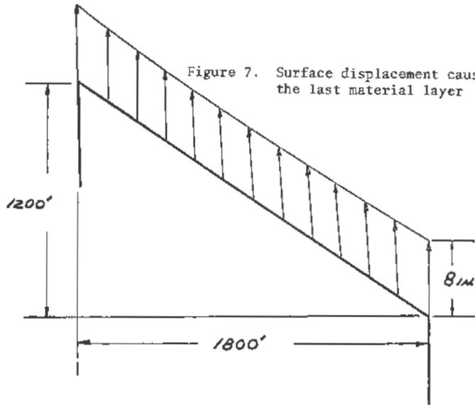
Figure 7. Surface displacement caused by the removal of the last material layer
