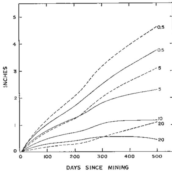
Figure 6. Development of vertical and horizontal creep around an opening 21 x 7.5 ft. in a mining panel in carnallitic potash. Dashed curves: Horizontal movement of pins anchored at distances as indicated. "Negative" movement of the vertical 20 ft. pin after 400 days indicates the recompression after initial stress relief creep due to pillar re-loading which resulted in increasing horizontal creep. For development of the vertical dimension of the creep zone as Figure 9.
