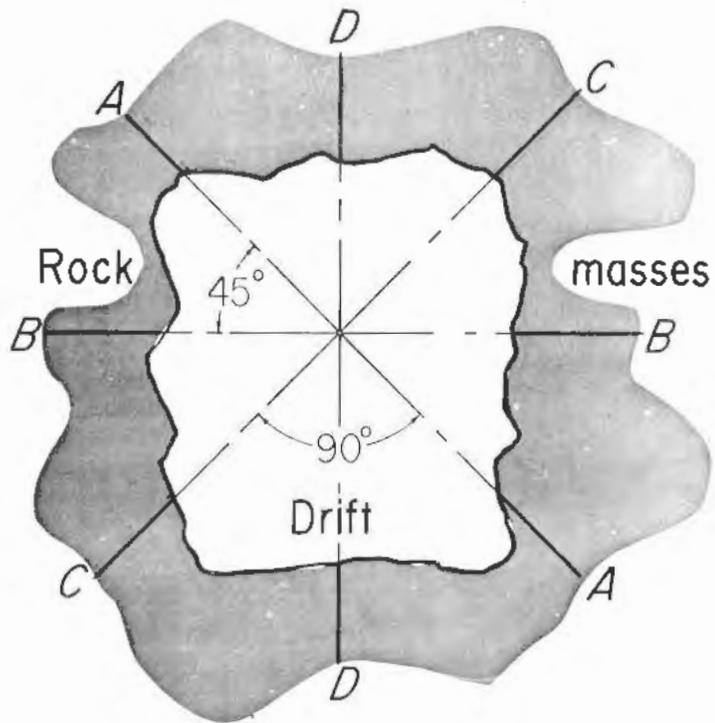
Figure 8. Orientation of measuring points
