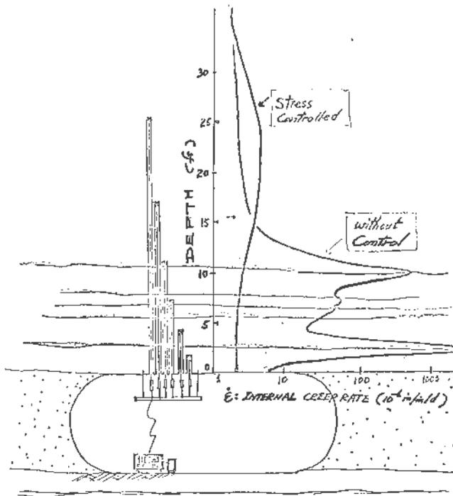
Figure 7b. Effectiveness of stress control shown by internal creep rate distribution.
