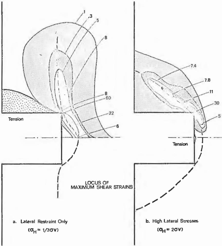
Figure 10. Shear strain contours around rectangular rooms.
