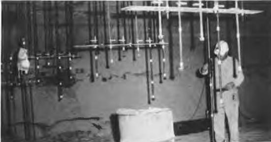
(a) Conventional creep station consisting of many anchor bolts measured by dial gauges
