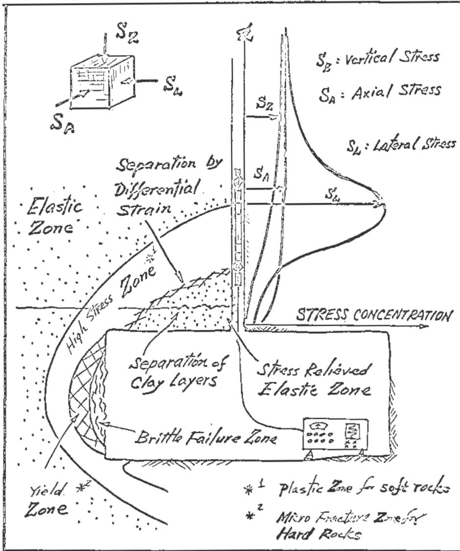
Figure 2a. General pattern of roof failure in bedded formations.
