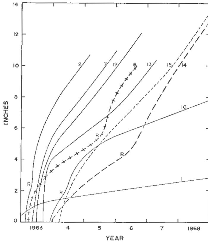
Figure 8. Vertical closure of rooms in relation to the development of the mined-out area shown in Figure 7. Creep curves identified with the same numbers for the respective locations shown in Figure 7.
