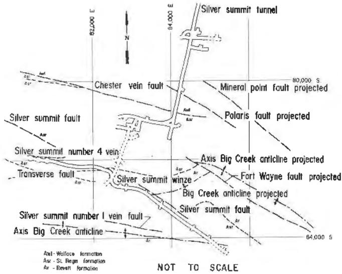
Figure 3. Structural geology, 4,000 level
