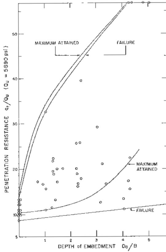
Figure 5. Penetration resistances observed in the tests at different depths of embedment
