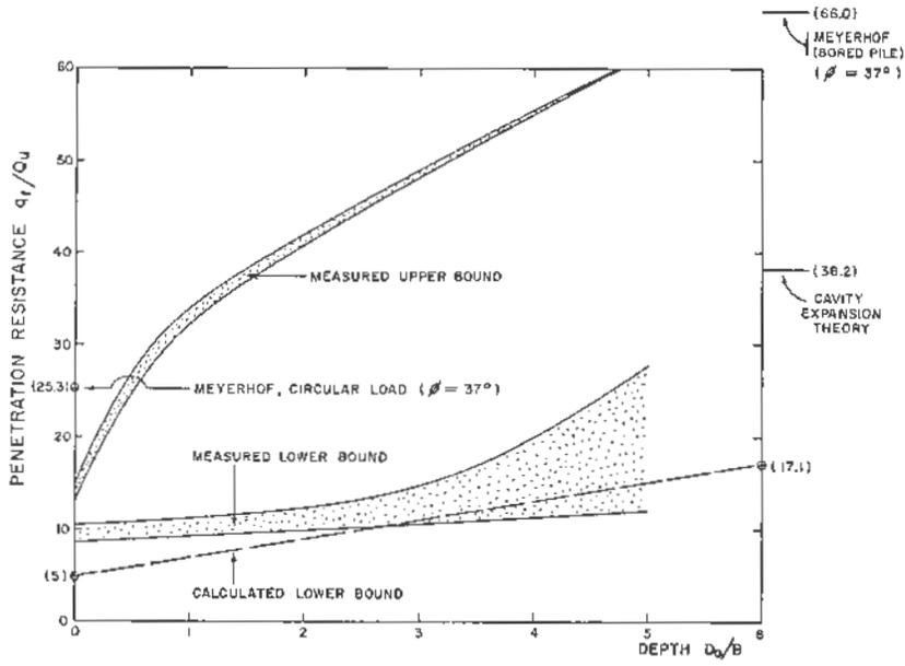
Figure 6. Comparison of experimental results with principal theories
