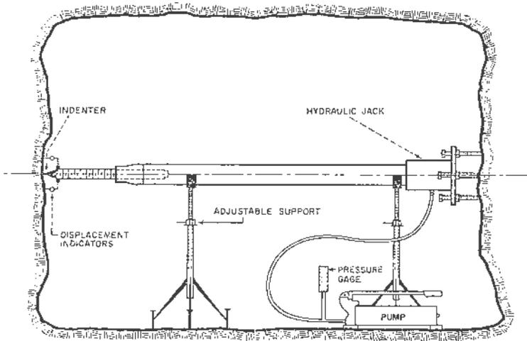
Figure 2. Schema of testing rig for bearing capacity tests
