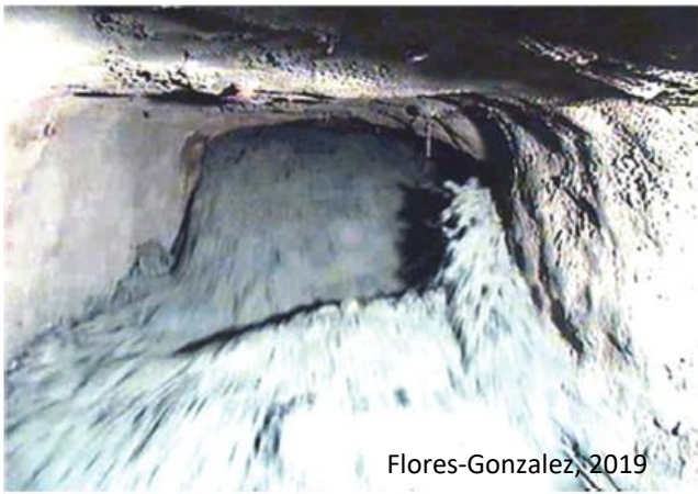
Inrushes of fines related to attrition of locally weak rock during drawdown
